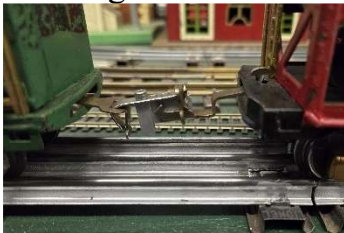
A.F. O Gauge with Slot & Hook
