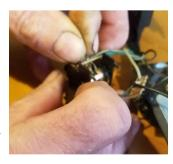
11.Retwist the tabs that hold the Contactor Plates in place. Just a little.
